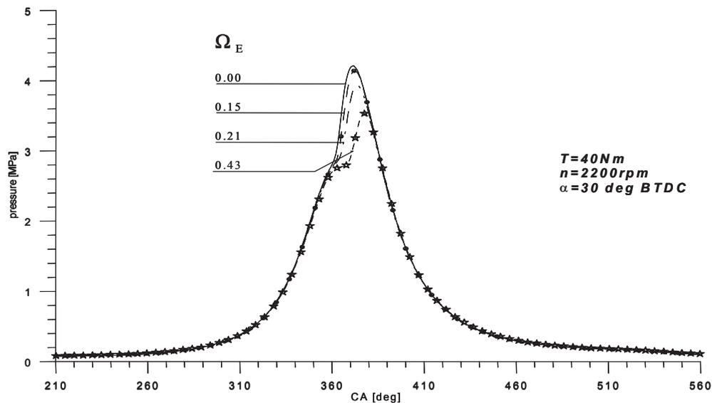
Fig. 11. Pressure vs. CA at high load, speed 2200 rpm and injection timing of RME = 30 CA deg BTDC for different ethanol fractions  $\Omega_E$ .
