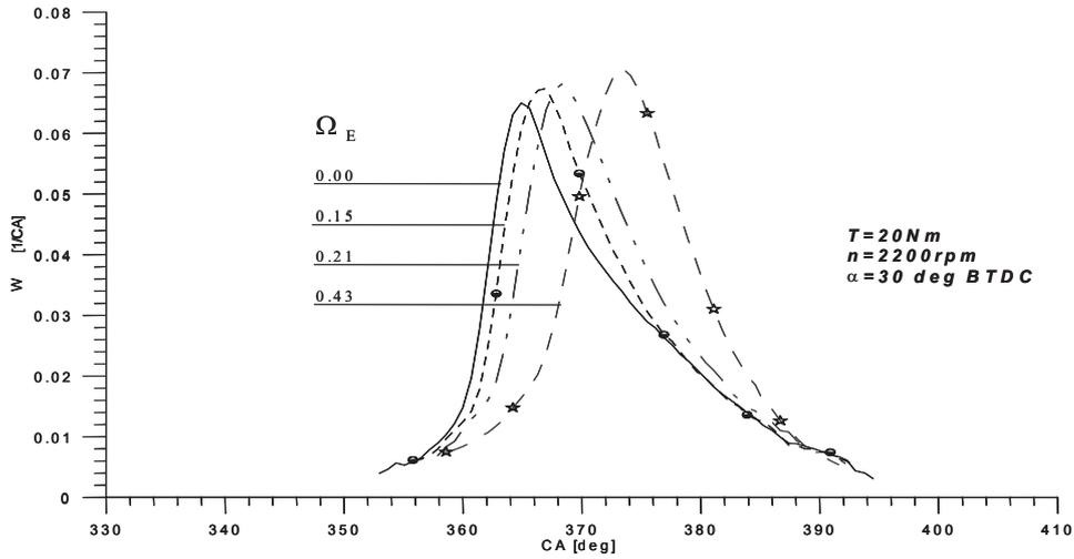
Fig. 12. Relative heat release rate vs. crank angle at low load and speed 2200 rpm for several ethanol energy fraction in total fuel  $\Omega_E$
