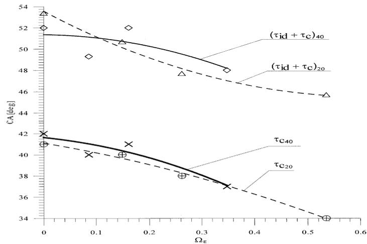
Fig. 16. Combustion time  $\tau_c$  [CA deg] and total combustion time  $\tau_{id} + \tau_c$  [CA deg] in function of ethanol energy  $\Omega_E$  at 1200 rpm and two loads
