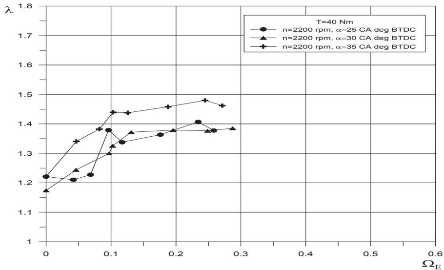
Fig. 9. Coefficient of air excess in function of ethanol energy fraction in total fuel for high load
