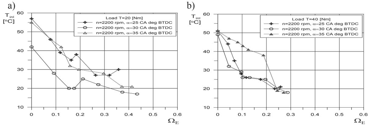
Fig. 2. Temperature of inlet charge in function of the ethanol energy fraction in total fuel at low load (a) and at high load (b)
