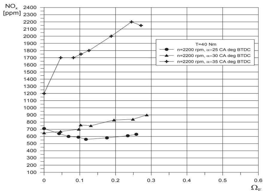
Fig. 4. Nitric oxide emission in function of ethanol energy fraction in total fuel for high load
