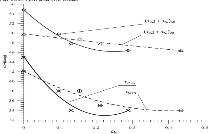
Fig. 18. Combustion time  $\tau_c$  [CA deg] and total combustion time  $\tau_{id} + \tau_c$  [CA deg] in function of ethanol energy  $\Omega_E$  at 2200 rpm and two loads
