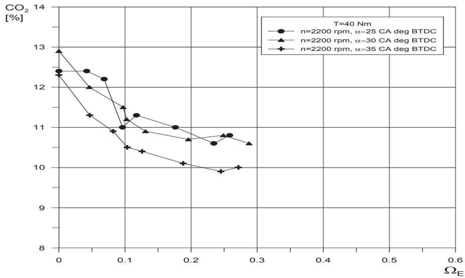
Fig. 5. Carbon dioxide emission in function of ethanol energy fraction in total fuel for high load
