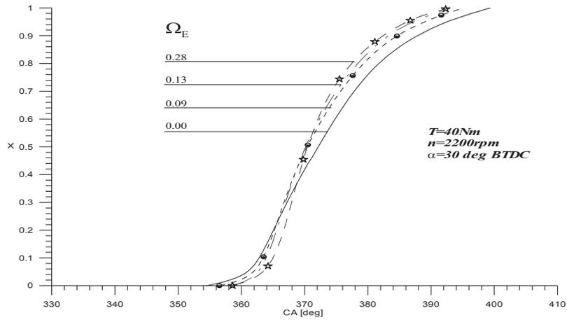
Fig. 15. Fraction of fuel burnt crank angle at high load and speed 2200 rpm for several ethanol energy fraction in total fuel  $\Omega_E$
