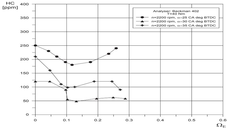
Fig. 8. Hydrocarbon emission in function of ethanol energy fraction in total fuel for high load
