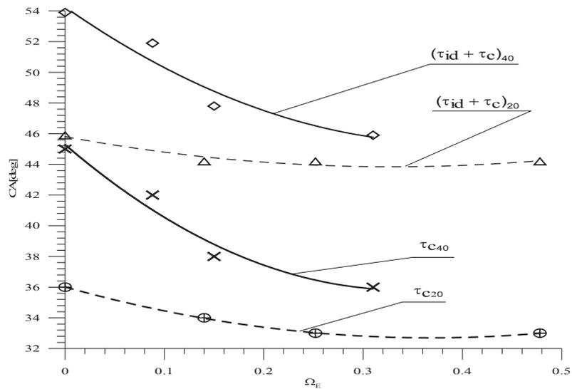
Fig. 17. Combustion time  $\tau_c$  [CA deg] and total combustion time  $\tau_{id} + \tau_c$  [CA deg] in function of ethanol energy  $\Omega_E$  at 1800 rpm and two loads
