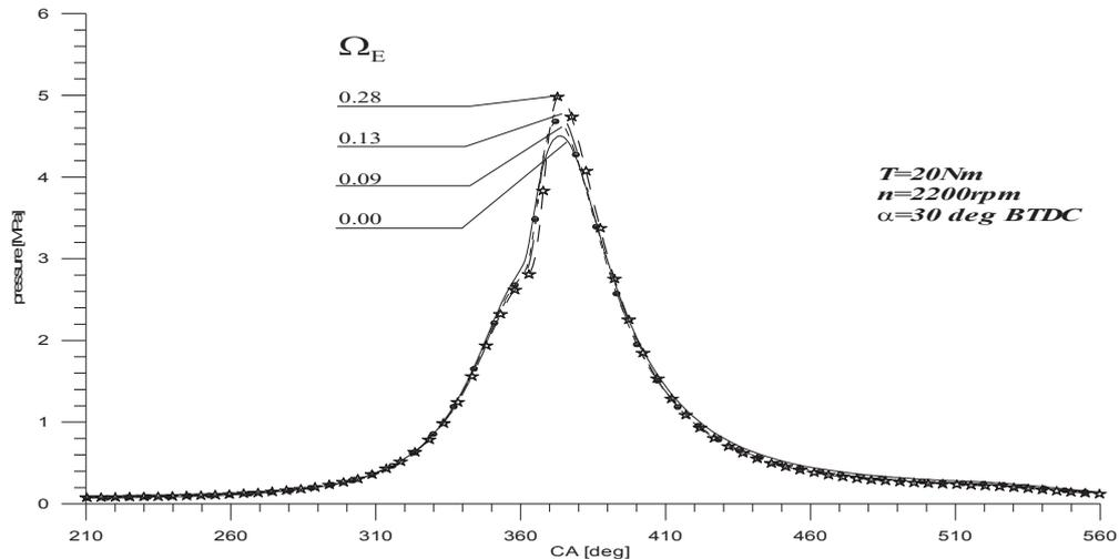
Fig. 10. Pressure vs. CA at low load, speed 2200 rpm and injection timing of RME = 30 CA deg BTDC for different ethanol fractions  $\Omega_E$ .
