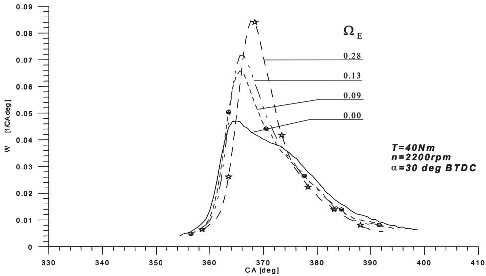
Fig. 13. Relative heat release rate vs. crank angle at high load and speed 2200 rpm for several ethanol energy fraction in total fuel  $\Omega_E$
