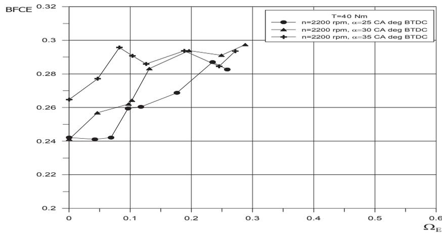
Fig. 3. Brake fuel conversion efficiency in function of ethanol energy fraction in total fuel for high load
