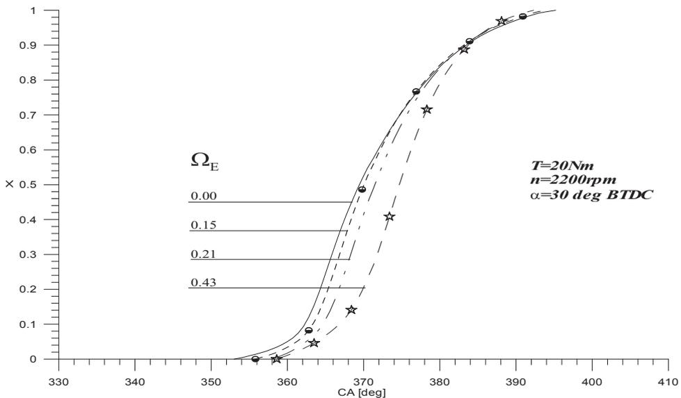
Fig. 14. Fraction of fuel burnt crank angle at low load and speed 2200 rpm for several ethanol energy fraction in total fuel  $\Omega_E$
