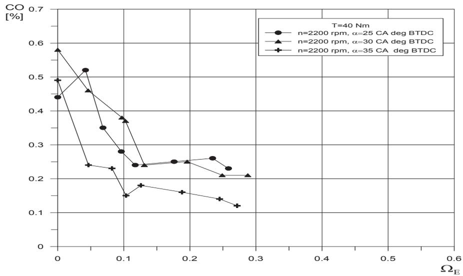
Fig. 7. Carbon monoxide emission in function of ethanol energy fraction in total fuel for high load
